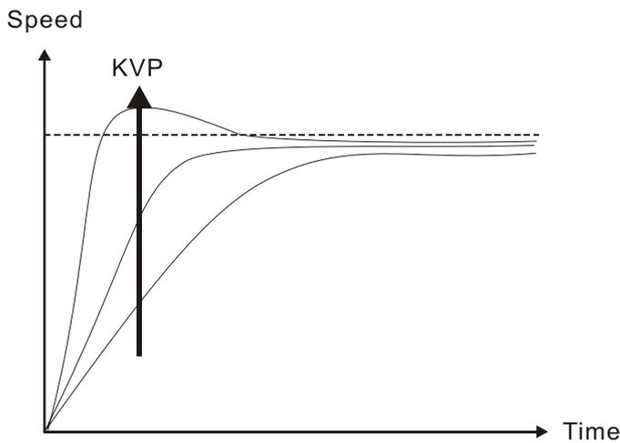
When the value of KVP is greater, the value of the responsiveness is also greater and the raising time is shorter. However, when the value of phase margin is over low, it is not helpful to steady error. But it is helpful to dynamic tracking error.
