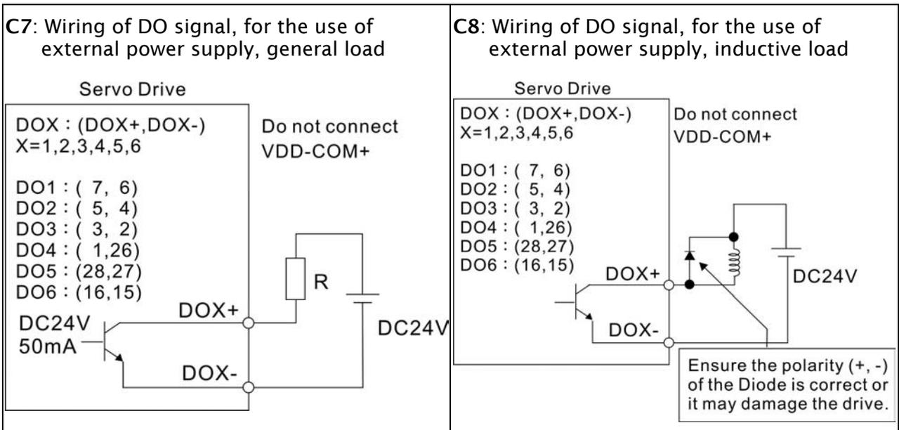
Use a relay or open-collector transistor to input signal.
