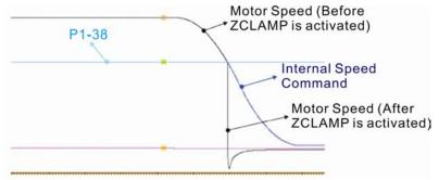
1: When the command source is an analog speed command, the users can use ZCLAMP DI signal to stop the motor at the desire position and do not care the acceleration and deceleration speed curve of the internal speed command. When ZCLAMP conditions are satisfied, the speed command is decreased to 0 r/min. When ZCLAMP conditions are not satisfied, the speed command will follow the analog speed command through Accel/Decel S-curve.
