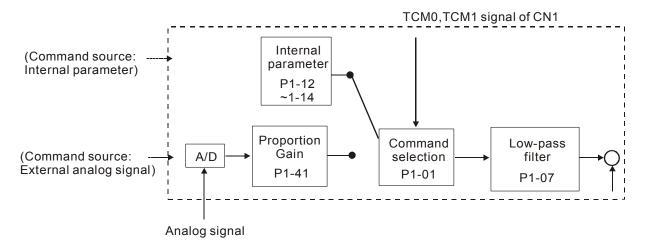
The command source is selected according to the state of TCM0, TCM1 and parameter P1-01 (T or Tz). Whenever the command signal needs to be more smoothly, we recommend the users to use proportional gain (scalar) and low-pass filter to adjust torque.
