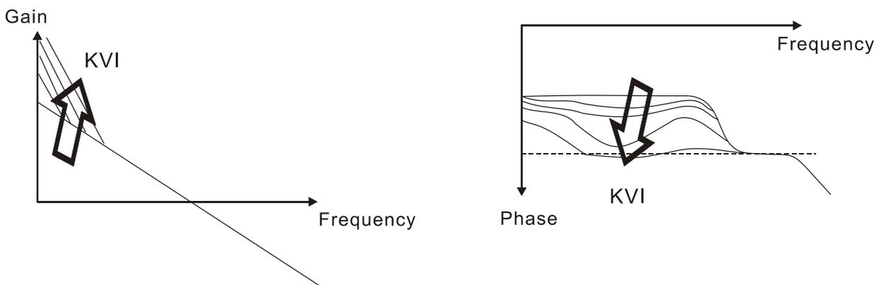
STEP 3 : Select the value of KVI, if the value of phase margin is too small, re-adjust the value of KVP again to obtain the value, 45deg of phase margin.
