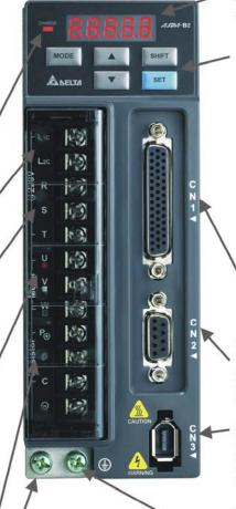
LED Display The 5-digit, 7 segment LED displays the servo status or fault codes.
