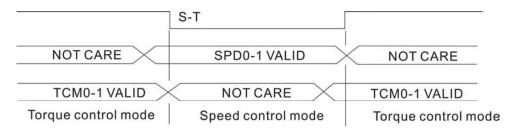
Figure 2.: Speed / Torque Control Mode Selection
