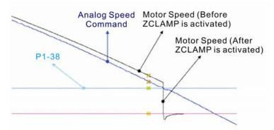
0: When the command source is an internal speed command, the users can use ZCLAMP DI signal to stop the motor at the desire position and keep the the acceleration and deceleration speed curve of the internal speed command. The motor will be locked at the position when ZCLAMP conditions are satisfied.
