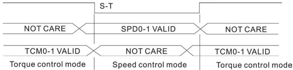
Figure 2. : Speed / Torque Control Mode Selection
