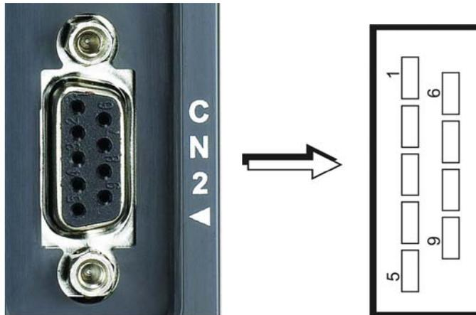
Figure 3.10 The layout of CN2 Motor Connector
