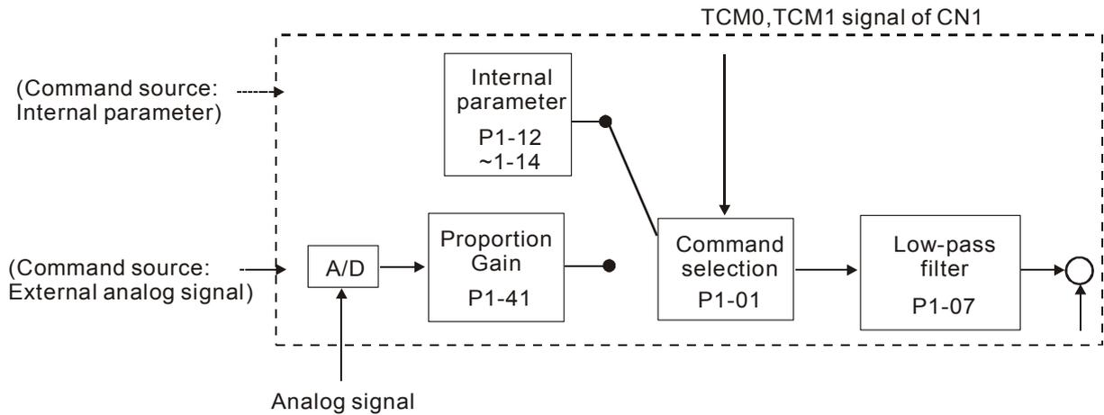
The command source is selected according to the state of TCM0, TCM1 and parameter P1-01 (T or Tz). Whenever the command signal needs to be more smoothly, we recommend the users to use proportional gain (scalar) and low-pass filter to adjust torque.
