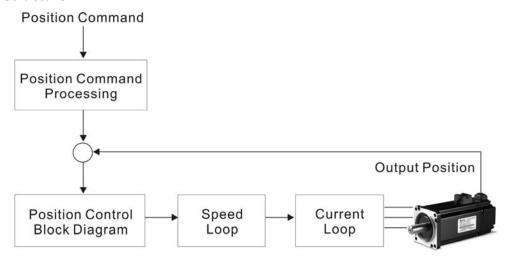
In order to pursue the goal of perfection in position control, the pulse signal should be modified through position command processing and the structure is shown as the figure below:
