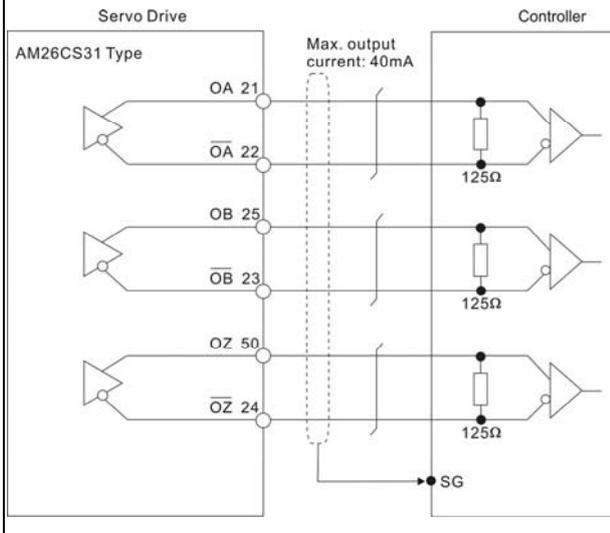
**C14: Encoder output signal (Photocoupler)**
