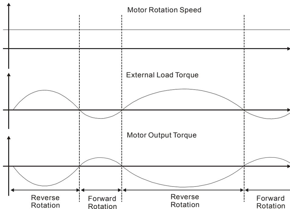
External load torque in reverse direction:  $T_L \times W_r$   $T_L$  : External load torque
