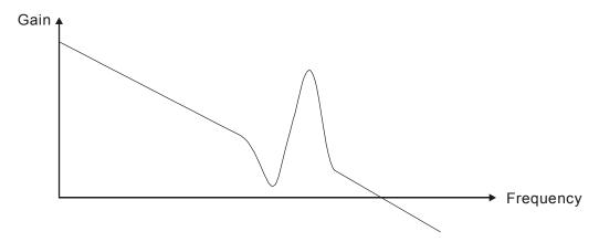
When the low-pass filter (parameter P2-25) is adjusted from 0 to high value, the value of Low-pass frequency (BW) will become smaller (see the figure below). The resonant condition is improved and the frequency response and phase margin will also decrease.
