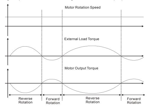
External load torque in reverse direction:  $TL \times Wr$  TL : External load torque For the safety, we strongly recommend the users should select the proper resistance value according to the load.
