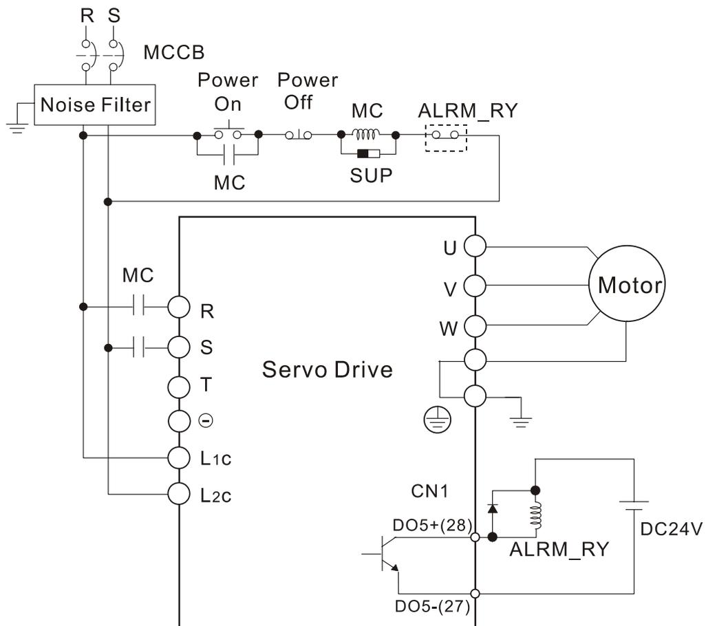
Figure 3.3 Three-Phase Power Supply (all models)
