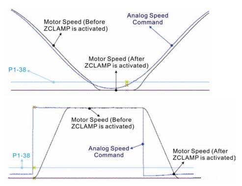
1: When the command source is an internal speed command, the users can use ZCLAMP DI signal to stop the motor at the desire position and keep the acceleration and deceleration speed curve of the analog speed command. When ZCLAMP conditions are satisfied, the speed command is forced to 0 r/min directly.
