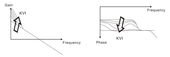
STEP 3: Select the value of KVI, if the value of phase margin is too small, re-adjust the value of KVP again to obtain the value, 45deg of phase margin.
