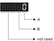
A: Analog monitor outputs polarity
