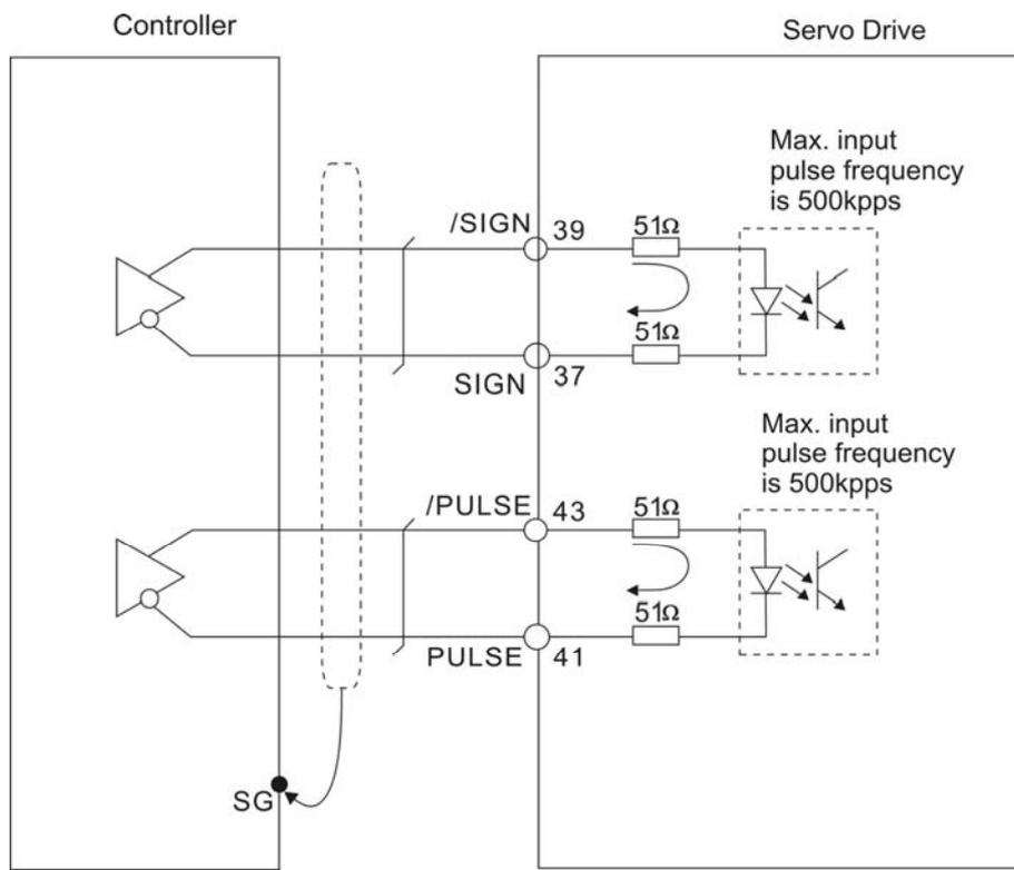
**C4-2: High-speed pulse input (Line driver)**. It requires 5V power supply only. Never apply a 24V power supply.
