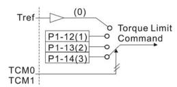
This parameter is used to determine that the speed and torque limit functions are enabled or disabled. If P1-02 is set to 11, it indicates that the speed and torque limit functions are enabled always. The users can also use DI signals, SPDLM and TRQLM to enable the speed and torque limit functions. Please note that DI signals, SPD0, SPD1, TCM0, and TCM1 are used to select the command source of the speed and torque limit.
