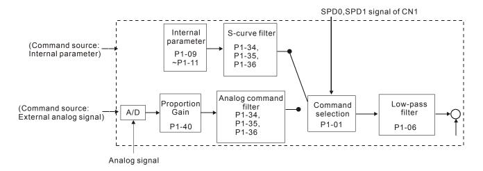
The command source is selected according to the state of SPD0, SPD1 and parameter P1-01 (S or Sz). Whenever the command signal needs to be more smoothly, we recommend the users to use S-curve and low-pass filter.
