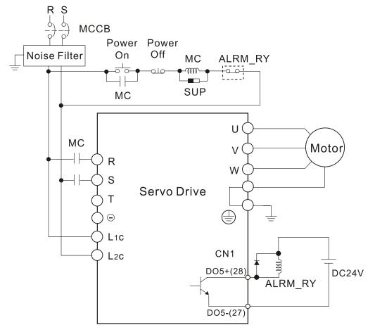
Figure 3.3 Three-Phase Power Supply (all models)
