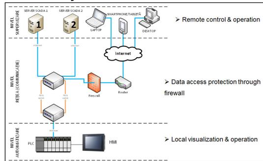
The **Control Layer** consists of 3 main AH-500 PLCs + I/O modules + DOP-B HMI → 1400 I/O points.
