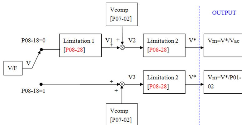
Limitation 1: IF  $V > Pr08-28 * (\text{Minimum of } VAC \text{ and } Pr01-02)$  then  $V = Pr08-28 * (\text{Minimum of } VAC \text{ and } Pr01-02)$
