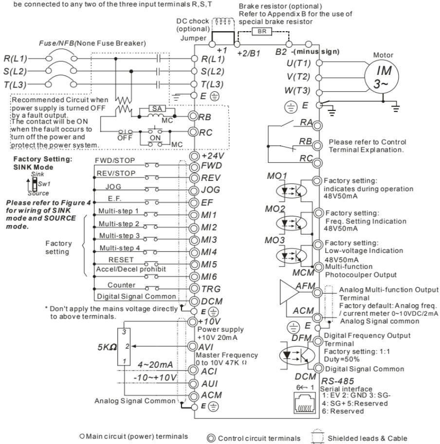
Figure 3 for models of VFD-B-P Series
