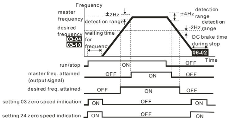
output timing chart of multiple function terminals
