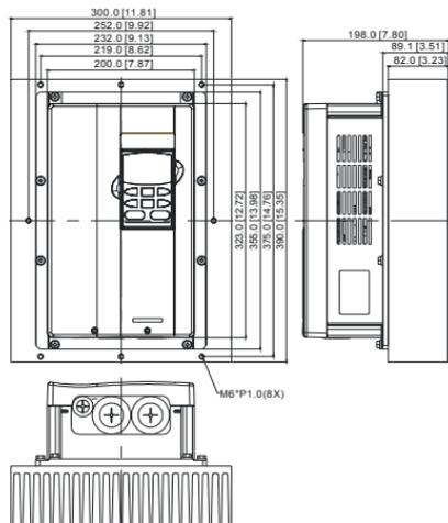
AC motor drive with heatsink MKB-PHC1
