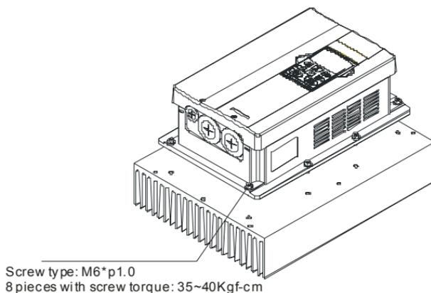
Heatsink (MKB-PHD/MKB-PHD1) for models VFD185B43P, VFD220B43P and VFD300B43P
