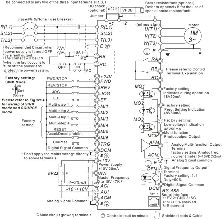
Figure 4 Wiring for SINK mode and SOURCE mode
