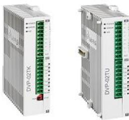
These DVP right side modules are specifically designed for temperature applications. There is no need to configure the communication as they are compatible with DVP-S series CPU. When many temperature loops are required in your application, you can connect 8 modules in a row and control up to 16 temperature loops in one single pack. This module not only can reduce the cabling and commissioning, but reduce the size of your control solution for sealing, glueing or heating/cooling applications.
